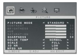
Picture Mode: Select the picture mode. you can choose "STANDARD,DYNAMIC, SOFT,USER" Contrast: Adjust picture contrast. Brightness: Adjust picture brightness. Tint: Adjust NTSC colour signal. Saturation: Adjust picture color. Sharpness: Adjust picture colour temp: cool, normal, warm mode. Scale Mode: Select picture scale. 3D NR:3D roise reduce, you can choose "Off,Low,Mid,High" MPEG NR:MPEG roise reduce, you can choose "Off,Low,High"
